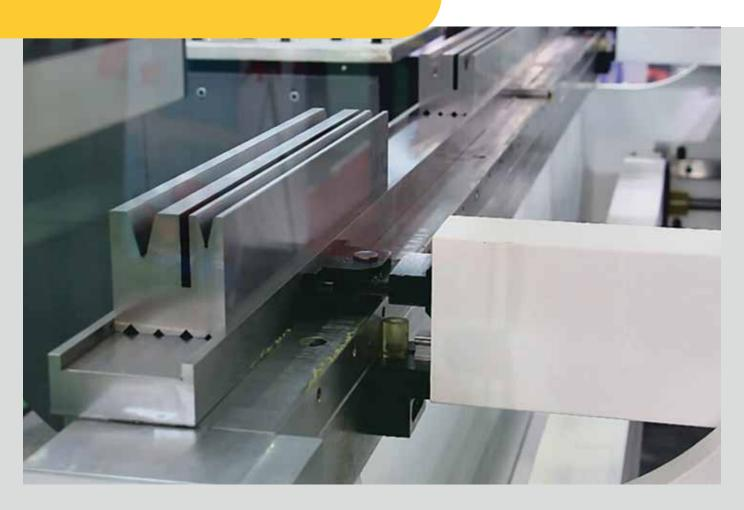
P1P2 Servo controlled table, to easy complete small bends, Using different V-openings in a die. Accurate positioning and reduced tool changes.
