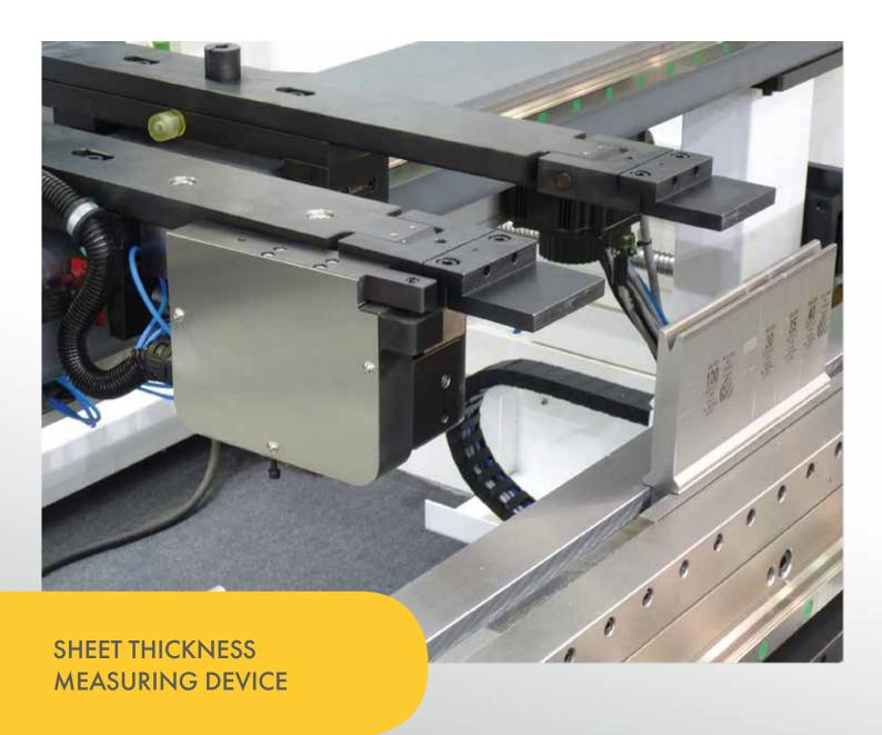
Automatic Sheet Measuring The "D-STM" sheet thickness measuring system is integrated in the backgauge finger. The D-STM measures the sheet thickness to an accuracy of +-0,0lmm, applicable up to 20mm of material thickness. The measuring cycle takes only tenths of a second, the measured data will be sent in real time to the CNC and the bending program will be adjusted.
