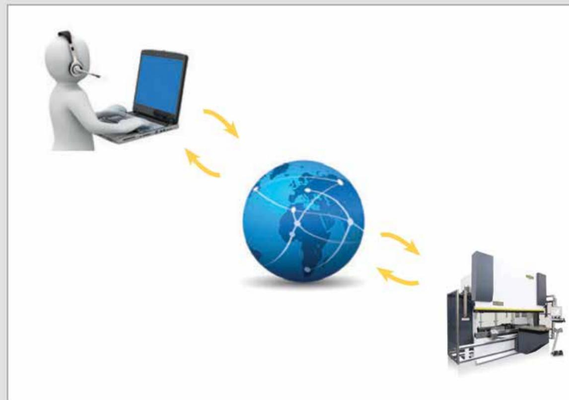
D-Remote Assistance is a feature of the ESA650, that allows a Deratech technician to temporarily log-on to the controller of the machine over a network or internet. This to provide help or resolve issues without directly touching the machine. This feature is simple to set-up, secure and only taking a few moments for our engineer to connect and begin the support session, resulting in time and cost saving solution for the end-user.
